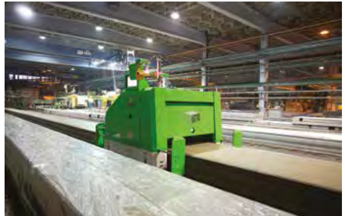
ABOVE: Elematic's automatic Plotter E9 for fast and accurate hollow core slab production.
