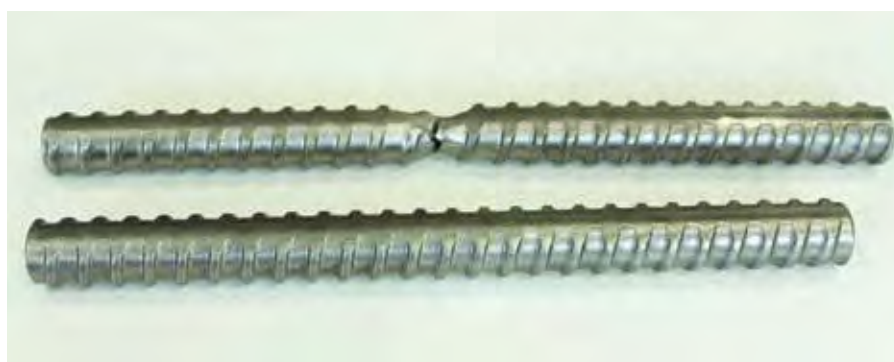
BELOW: The high ductility of SAS ULTS exceeds the requirements of the standard for low temperature applications at -165°C (more than 3%), and it has the same ductility at -165°C as a standard reinforcement bar at ambient temperature.
