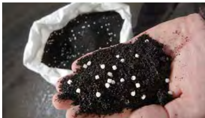
ABOVE AND BELOW: Vestenamer by Evonik makes it feasible to process rubber powder from scrap tyres to generate asphalt with rubber content. The recycled material is mixed into road construction bitumen or asphalt to improve the quality of the mixtures and to extend the service life of road surfaces.
