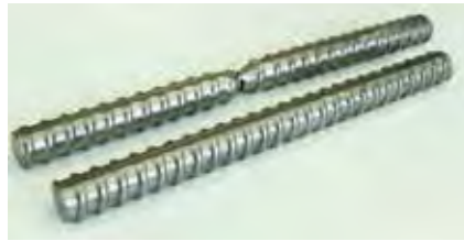
ABOVE: The SAS ULTS are manufactured in diameters between 12 mm and 32 mm, cross sections ranging from 113 sq mm to 804 sq mm, and yield loads of 57 kN to 402 kN.
