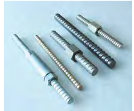
ABOVE: The SAS ULTS are manufactured in diameters between 12 mm and 32 mm, cross sections ranging from 113 sq mm to 804 sq mm, and yield loads of 57 kN to 402 kN.
