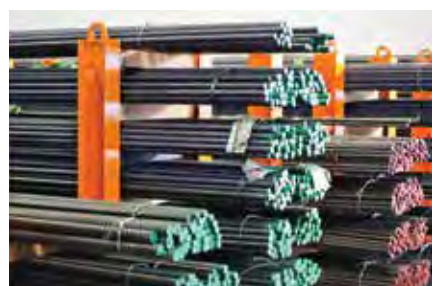
SAS Asia warehouse in Singapore stores up to 1,000 t of SAS fully threaded bars and accessories of different grades and diameters.
